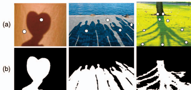
Fig. 18. Examples of user-guided extraction of shadow masks based on region growing and SVM. (a) Shadow images. The circles signify the supplied shadow and nonshadow observations. (b) Shadow masks extracted using region growing and SVM.
